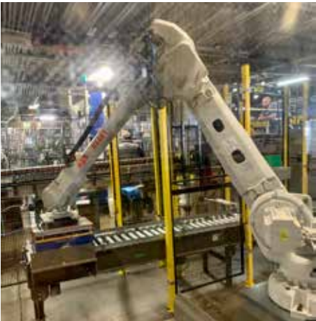
We installed a new palletizer to reduce employee risk of injury from lifting and stacking. The robot has been named “Haagy” after a beloved long-time co-worker who passed away in 2019.
